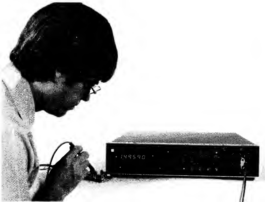
Figure 7-1. Hewlett-Packard Model 3455A Digital Voltmeter designed for both bench and systems applications
