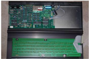
When fitted internally, the MAGROM PCB is mounted with the components facing downwards.
