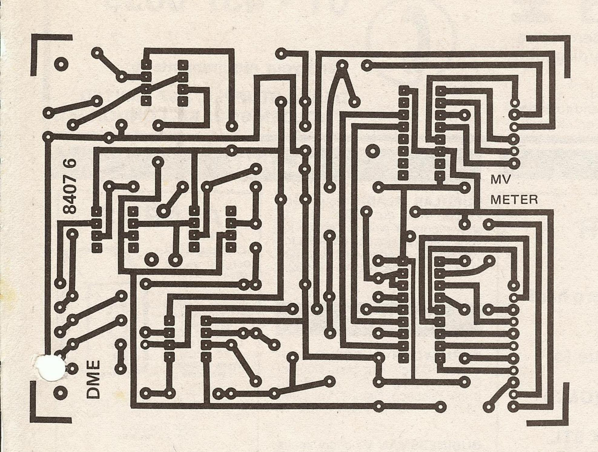
To the left is the foil for the Audio/Millivoltmeter project. Below is the pattern for the Memotech Echo unit.
