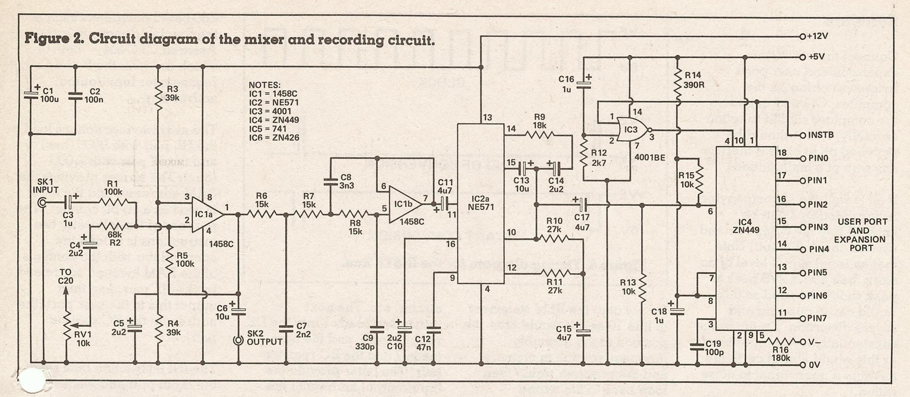
Power for the unit is taken from the expansion port at the left hand side of the computer. This requires a 2 by 30 way 0.1 inch pitch edge connector with the appropriate polarising key. In practice it is unlikely that a suitable connector will be available, but the connections can be made via a Spectrum type, 2 by 23 way 0.1 inch pitch edge connector.
