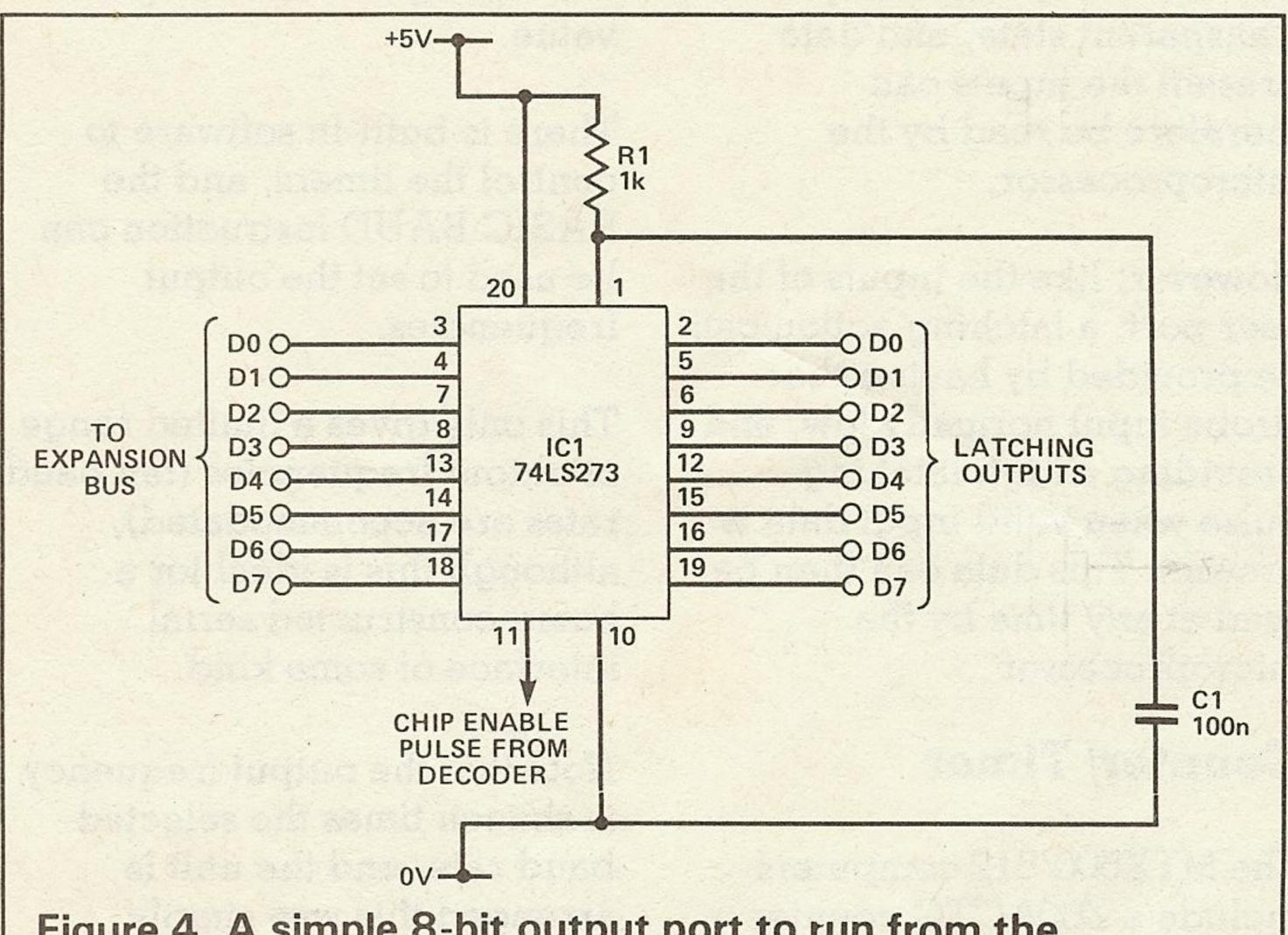
Figure 4. A simple 8-bit output port to run from the expansion bus.
