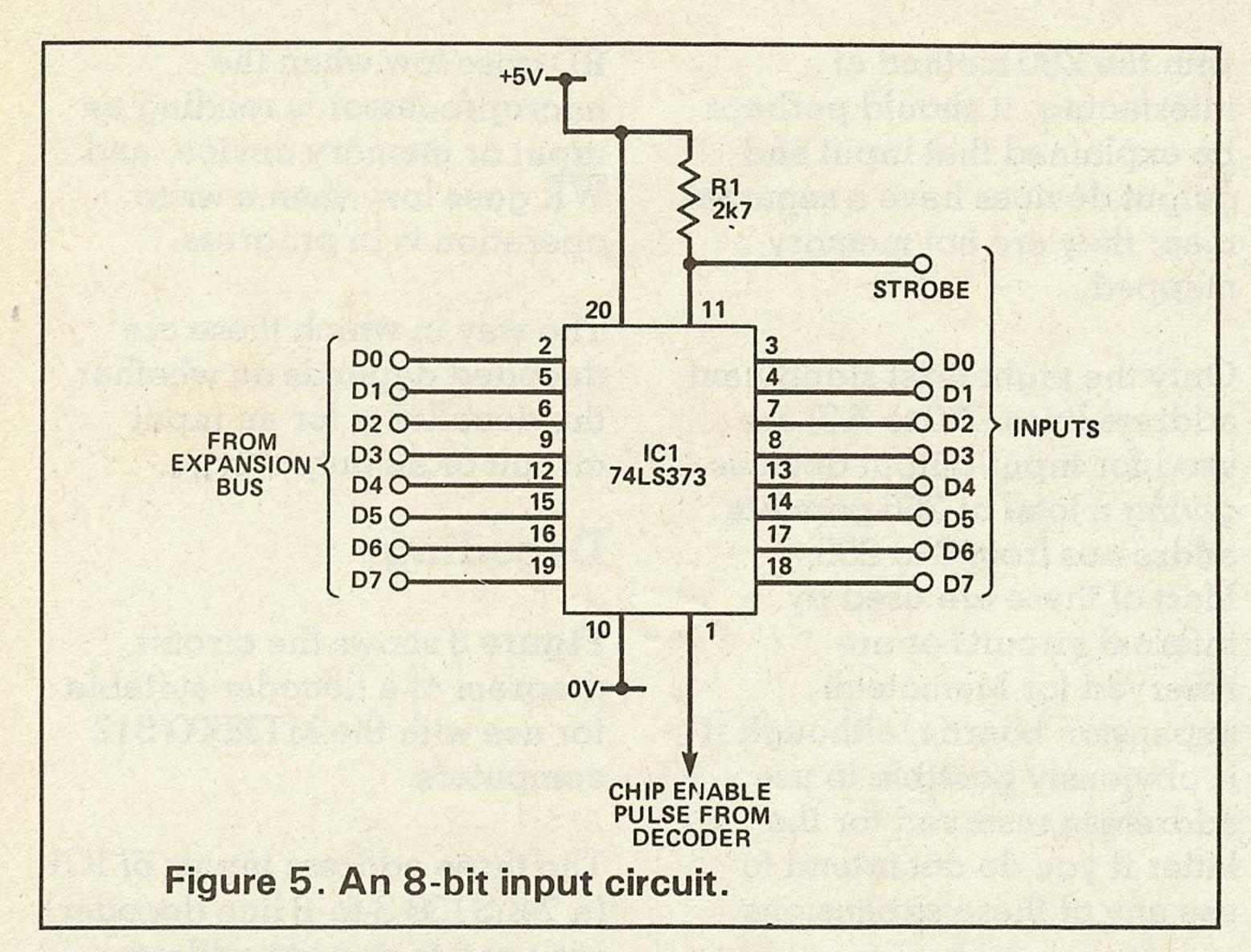
ICI is an octal D-type flip/flop which is used here as an octal latch with the latching pulse from the decoder being applied to the clock input.
