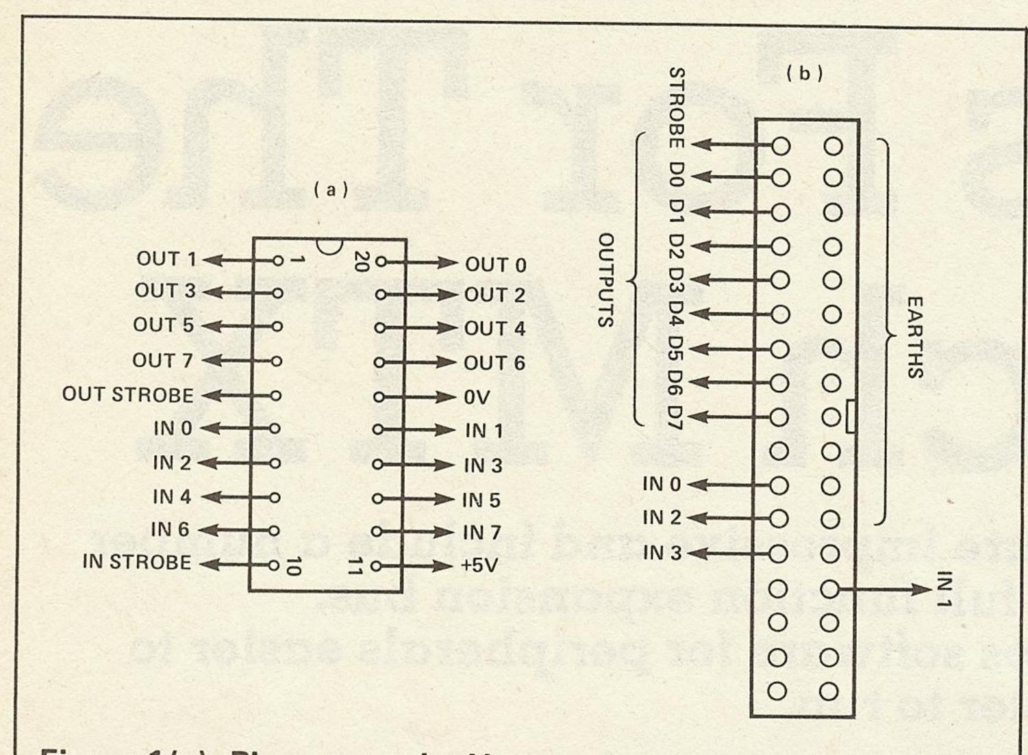
Figure 1(a). Pin-outs at the User port, a dedicated I/O socket. Figure 1(b). Details of the printer port.
