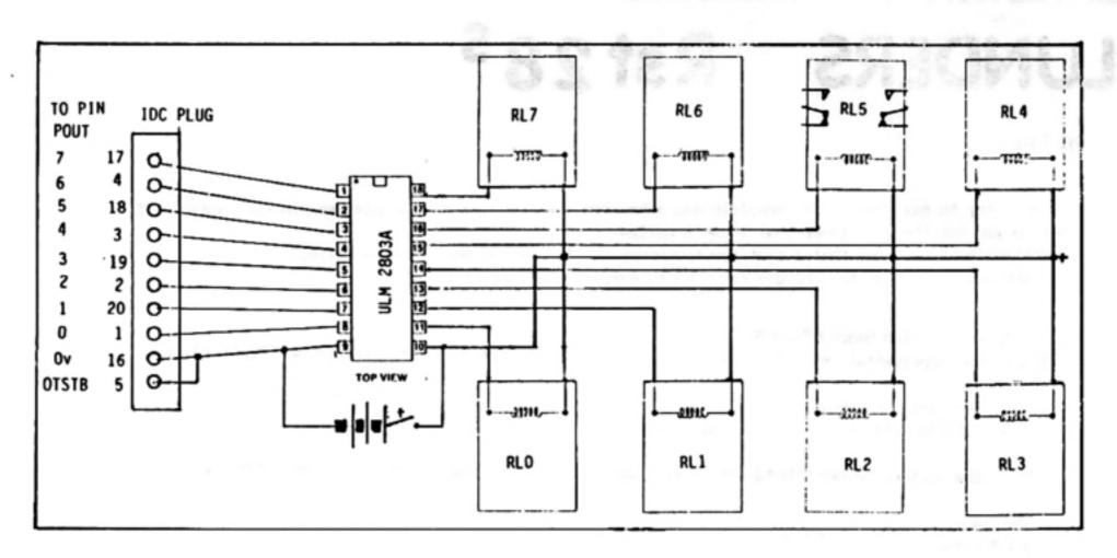
The circuit which is shown below was constructed on a Vero V Q Board designed for dual-in-line circuits. (Maplin HQ 48C). This is a good base in many respects and is ideal for relay mounting but does need a large number of interconnections on the top of the board. The relays were soldered directly to the board but an 18 pin DIL socket (Maplin HQ 76 H) was used to mount the I C chip.
