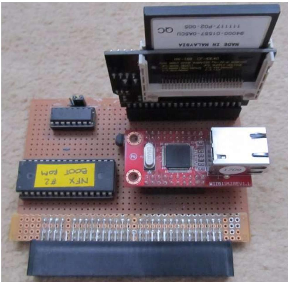
With the CF and ethernet module removed, the minimal nature of the design is readily apparent. The only logic device on the board is a 74HC138. The WIZ5100 is a 3.3 volt device, so there is a 3 pin LDO to supply the 3v to the module, plus pull up resistors for the module SPI pins.
