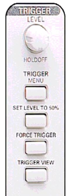
Figure 5: Trigger Controls
