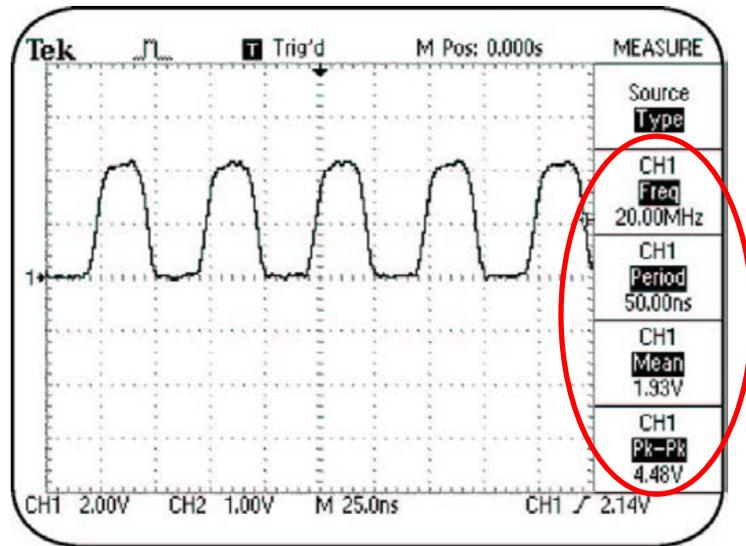
Figure 6: Example of automated measurements with digital readouts.
