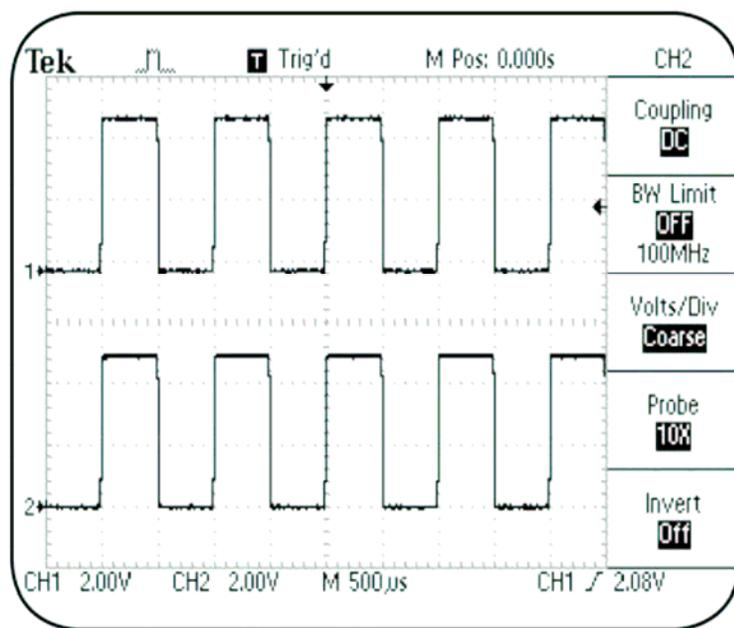
Figure 2: Example of a two-trace display on the TDS 220.
