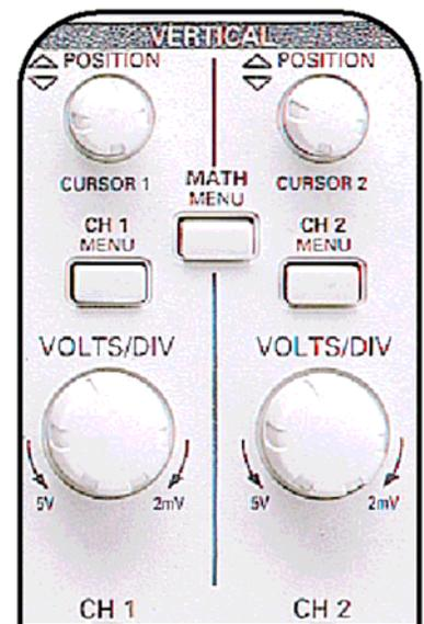
Figure 3: Vertical Controls.
