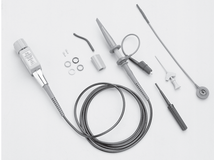
Figure 2.15. A typical general-purpose voltage probe with its standard accessories.
