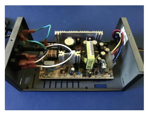
You can then screw the lid of the enclosure back in place and fit the upgraded power supply unit back inside the TC01.
