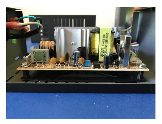
Now the mains power cables can be attached from the switch to the poles on the power supply, with the earth cable connected from the free spade connector on the enclosure to the power supply. Next, connect the Molex 6 pole housing from the computer power loom made above to the output pins. It's worth placing a self-adhesive cable tie mount on the inside of the enclosure so that the
