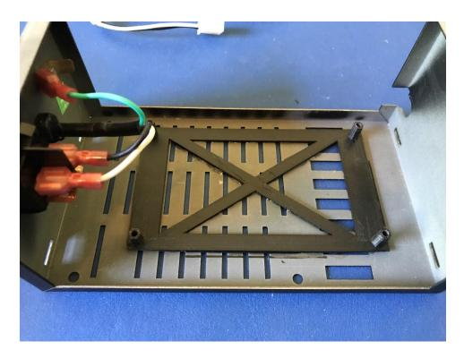
The mounting plate edges were curled slightly, so extra care is needed to make sure that yours doesn't suffer from the same issue. In my case, it didn't affect the mounting of the power supply or its adhesion to the base of the enclosure. The power supply is mounted in place using four M3 screws.
