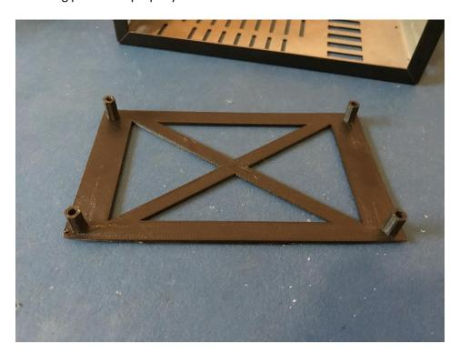
Secure the base of the printed mounting plate to the base of the enclosure using epoxy glue taking care not letting it seep out of the ventilation grilles. Mounting it off centre allows clearance for the mains cable to the switch and the mains power cables from the switch to the power supply.
