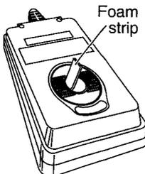
Before using the mouse, remove the packing material. Turn the mouse upside down and pull out the foam strip that holds the mouse ball in place.
